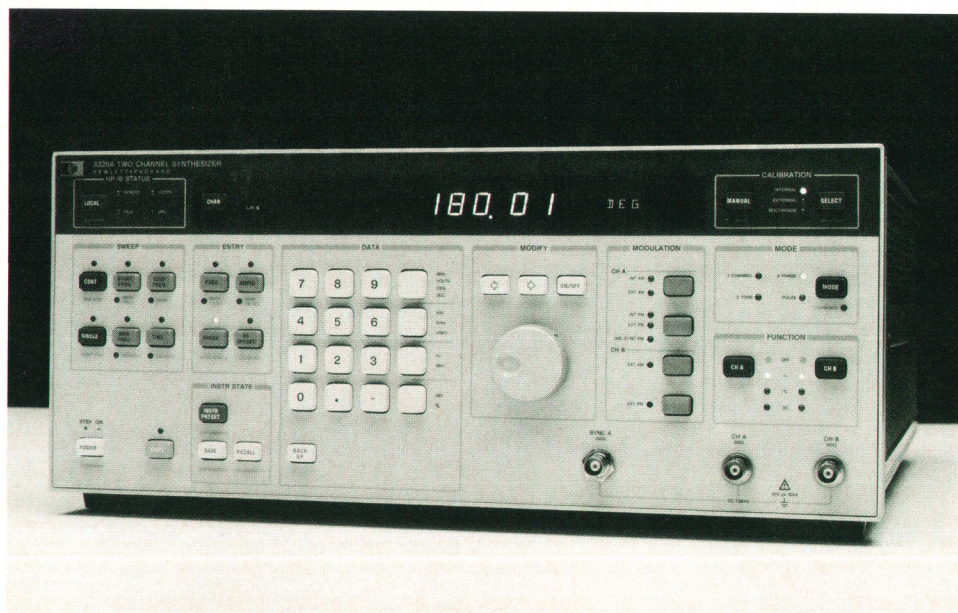
Fig. 1. The HP 3326A Two-Channel Synthesizer can generate either two independent signals or a combination of the signals in its two channels. Each channel produces sine and square waves from 1 \mu Hz to 13 MHz with separately controllable amplitude and dc offset. Pulse and flexible modulation capabilities are built-in.
